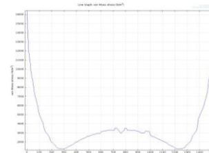
Figure 4.7 shows the stress distribution in the cantilever at the input edge.
